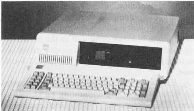
Fig. 1-4. The system unit sits behind a detachable keyboard.
